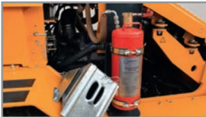
Fire Fighting System
