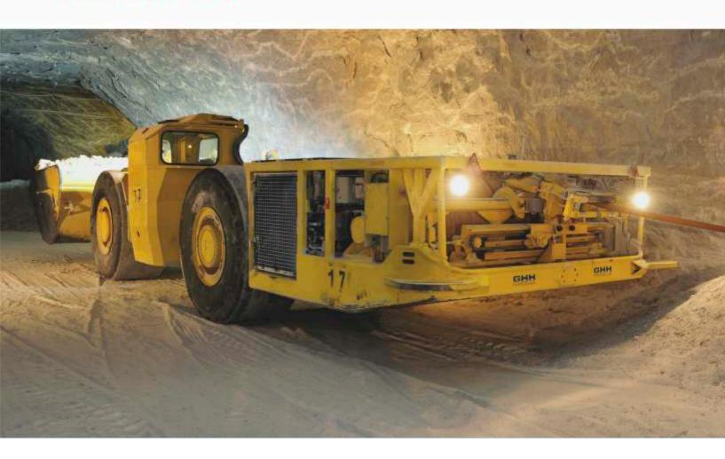
GHH offers electric LHD with capacities up to 19 tons. Furthermore, all electric LHDs are equipped with an active drum control which ensures an orderly winding, whereby a long service life of the cable is reached due to low tensile forces.
