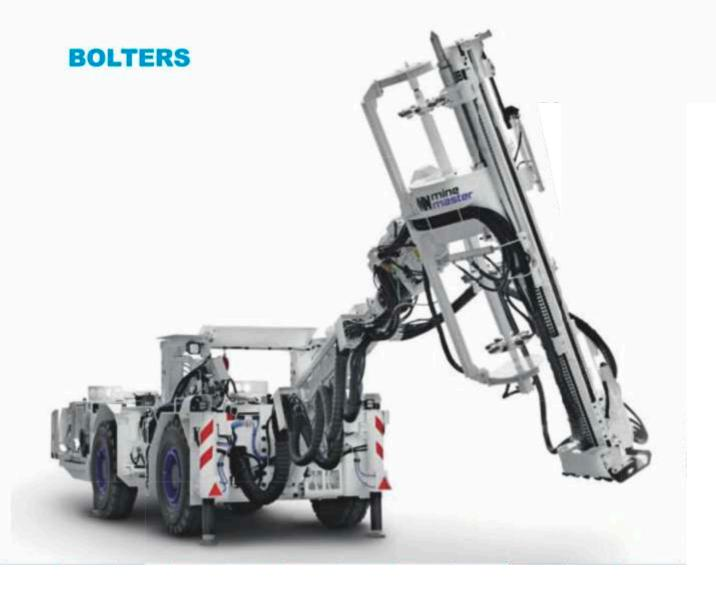
Roof support in mining excavations and tunnels by means of roof-bolting is one of the applications that can be achieved by machines manufactured by our company. Self-propelled bolting rigs featuring various parameters depending on the height of the roof and hardness of rock are manufactured to tailor individual clients applications.
