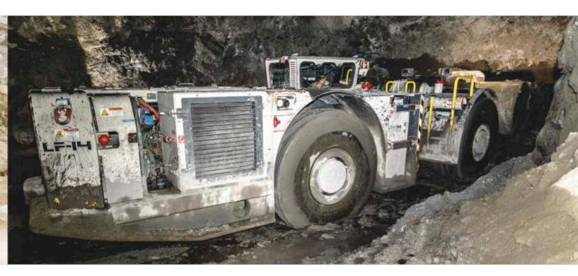
GHH Diesel LHDs are custom designed to operate in the narrow vein and midseam mass mining operations. They are efficiently compact with an optimal operator's position. The lateral arrangement of the operator seat guarantees optimal views for forward and backward tramming. The capacities of the GHH LHDs are ranging between 1 to 21 tons. The LHDs are globally used in underground mining, in tunneling, hydro-power and other civil construction projects.
