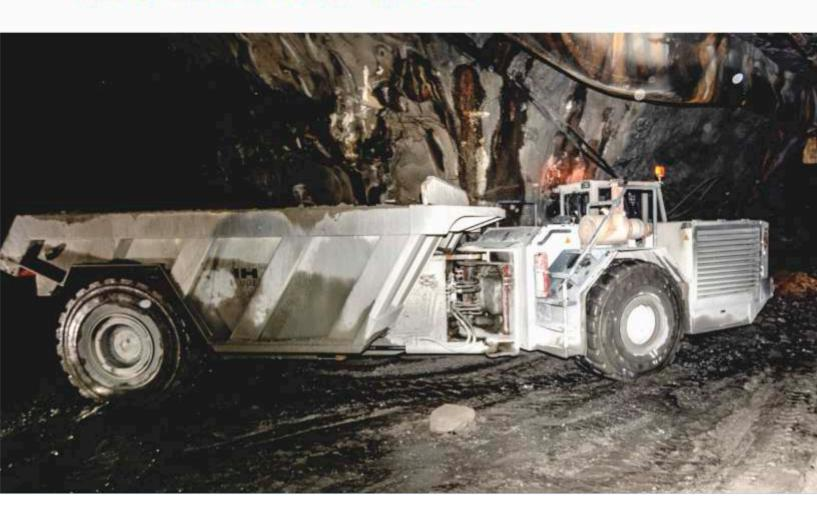
GHH Group manufactures articulated dump trucks for mining and tunneling with capacities from 20 to 45 tons, and bowl sizes from 6 to 24m³. Our vehicles are characterized by their compact dimensions, higher comfort and better maneuverability with a swivel hinge. The vehicles have an excellent power to weight ratio to ensure high speeds even in high gradients. The particularly basic and robust design of the vehicles ensures a long service life at low operating costs.
