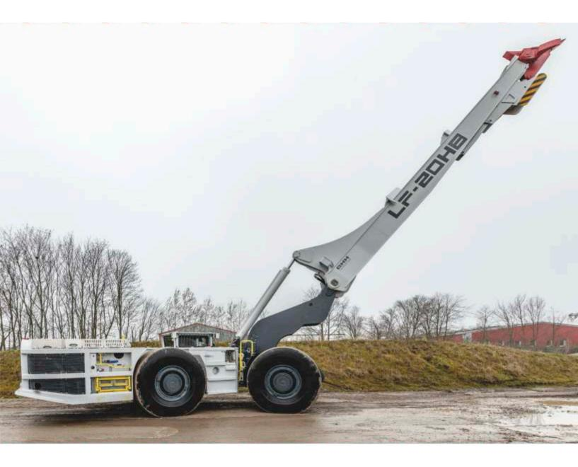
Based on standard LHDs GHH also offers shearing scalers to prepare the roof for subsequent roof support. The highly efficient working principle of our shearing scalers is combined with the proven hydrostatic drive train EDS, which allows for sensitive roof and side wall scaling as well as quick reversing.
